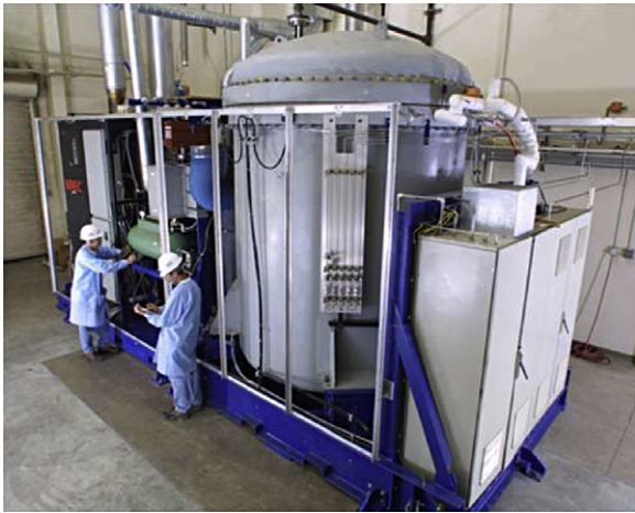
Fig. 1. Pressurized 220 kW SOFC/GT hybrid system.
